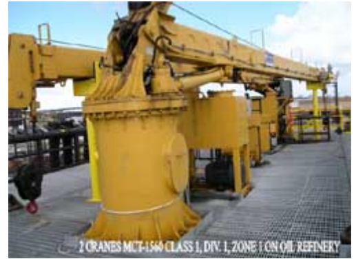
15T telescopic crane, class 1 div 1 zone 1 on oil refinery
