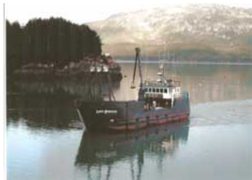
Alaska Marine Crane © 12T knuckle boom crane on fishing vessel
