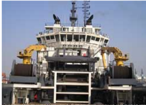
2 OFFSHORE CRANES MCK-2552 ON TIDEWATER ANCHOR HANDLING TUG 2 offshore cranes, 25T knuckle cranes on AHT
